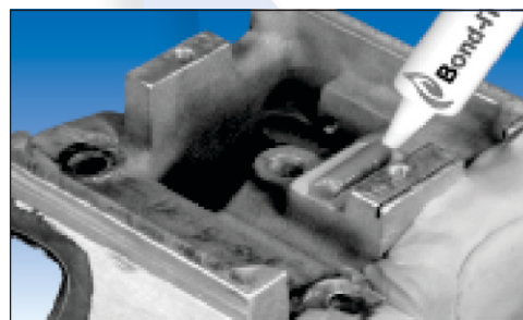
Bond-IT™ 7056AL Fills a Casting Before Re-Machining
